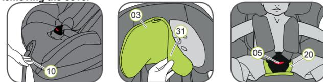
1. Press the recline handle (10) upwards and slide the seat shell (18) to the rear into the upright position.
